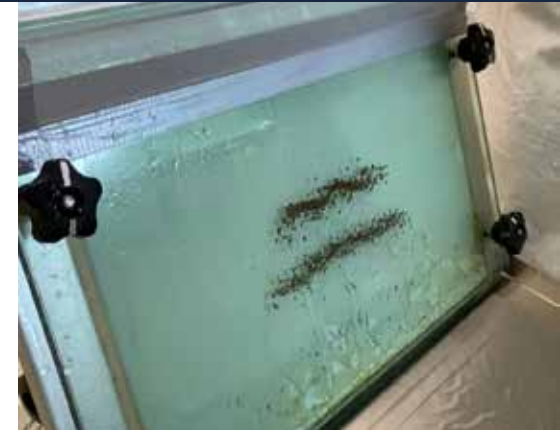
Manual male and female pupae separator - hock sorter
