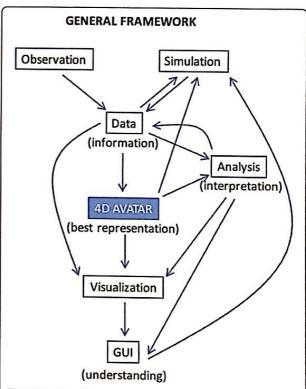
Fig. 1 The data-driven avatar communicates knowledge through a Graphical User Interface (GUI) customized for different stakeholders. Their improved understanding in turn generates new hypotheses to test and new simulations to run, thus driving further data collection
