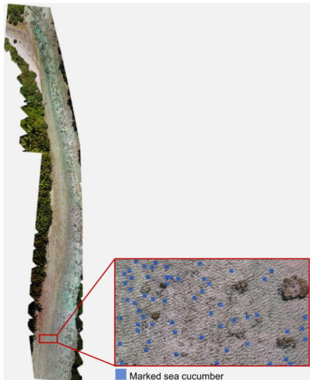
Figure 4. Photomosaic map of study region in Tetiaroa, French Polynesia generated by stitching 57 overlapping, geo-referenced images using the application Pix4DCapture. Inset highlights a zoomed in portion of image with sea cucumbers manually marked using Visual Counter.
